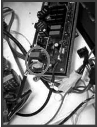
5-Remove 2 wires of Ballast module (PWB).
