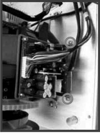
1.-Screw off 2 screws of LVPS PWB.
