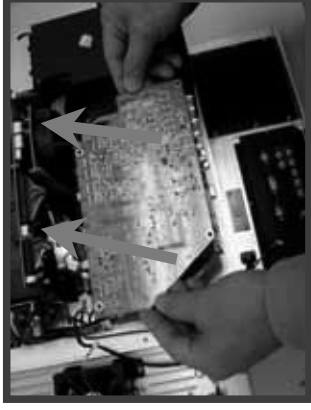
4-Pull up the RCA PWB vertically.
