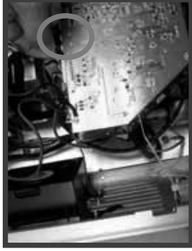
3.-Disconnect 1 cable from right panel.
