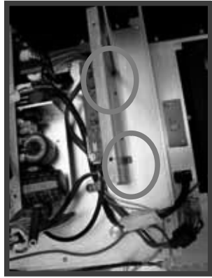
4.-Screw off 2 screws of Ballast module (PWB).
