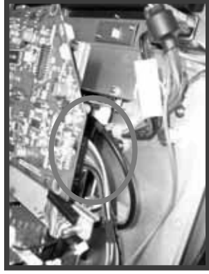
7-Disconnect 1 cable of the Main PWB.
